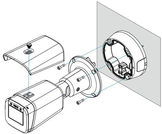
12 Band the stand to adjust the camera angle accordingly. For details, refer to the **Angle Adjustment**.
