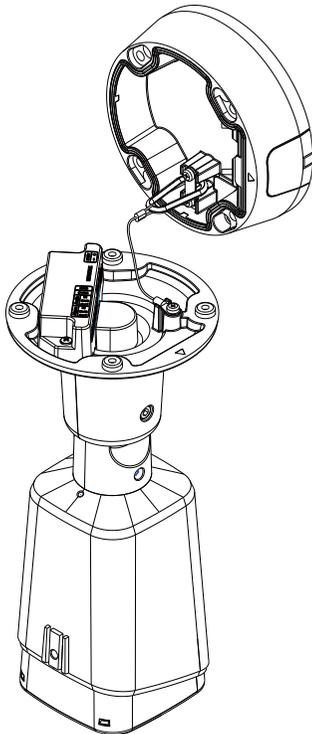
9 Connect the alarm, network and power adapter.
