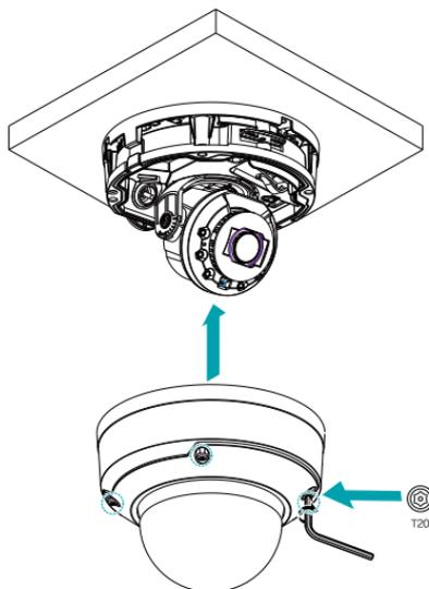
Remove the protective film inside and outside before closing the dome cover.
