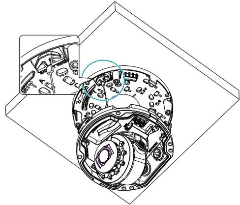
7 Attach the camera body to the installation bracket by rotating it clockwise as shown below. You will hear a click when it is properly mounted.
