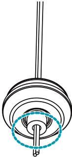
3 Assemble the cable rubber to the camera body.
