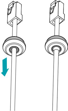
If you insert a thin cable or more than two cables, it is advised to finish by using silicon to make sure to perfectly waterproof it. (Silicon finishing part — refer to the bottom image.)
