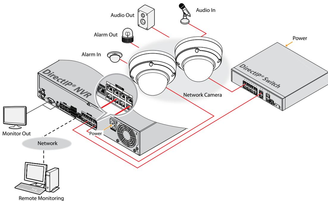
DirectIP® NVR makes it easy to use cameras without extra network configurations. Each camera can be controlled via the DirectIP® NVR setup menu, without any PC. For detailed camera settings, please see the camera setting pages of DirectIP® NVR manual.
