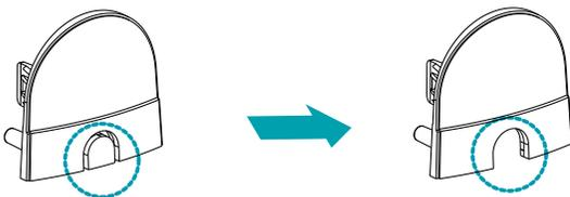
2-2 Insert the LAN cable through the cable rubber using the protect connector.
