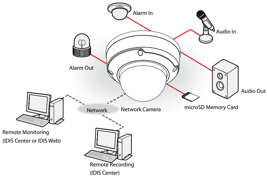
Control the camera over the network from software installed on a computer.
